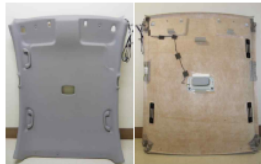
Fig. 4. Module of headliner made from a 50/50 PLA/kenaf fiber biocomposite.
