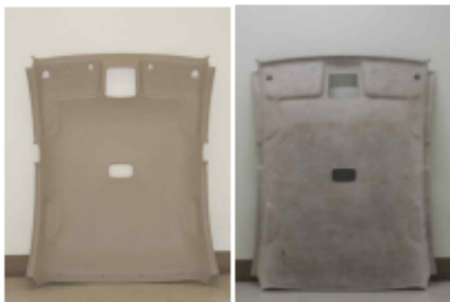
Fig. 2. Prototype headliner composed of PLA/kenaf fiber bio-composites.
