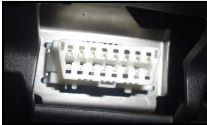
**Figura 3.17.**Conector OBDII.
