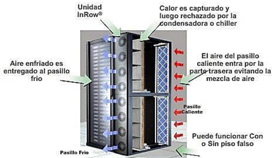
**Figura 4.7** Esquema Close-coupled cooling
