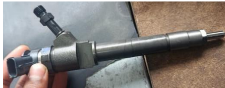
Figura 2 Injector Diesel Common Rail – Vista Lateral
