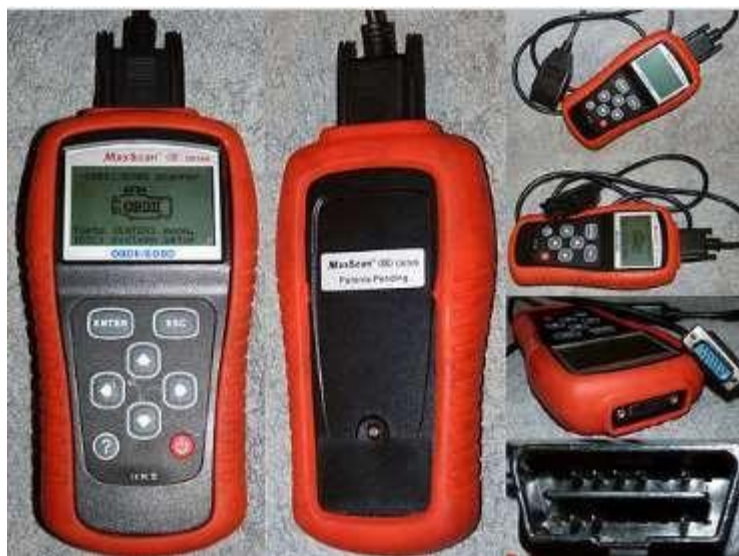
Figura 7: On Board Diagnostocs II – OBD2
