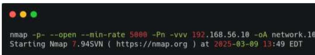
A terminal window with a dark background. The command executed is `nmap -p- --open --min-rate 5000 -Pn -vvv 192.168.56.10 -oA network.10`. The output shows the start of the scan for 192.168.56.10 at 2025-03-09 13:49 EDT. The terminal title bar shows the path `~/goad/nmap`.
