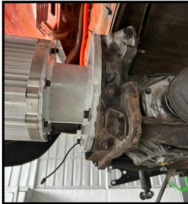
**Figura 7.17:** Acople Caja-Motor
