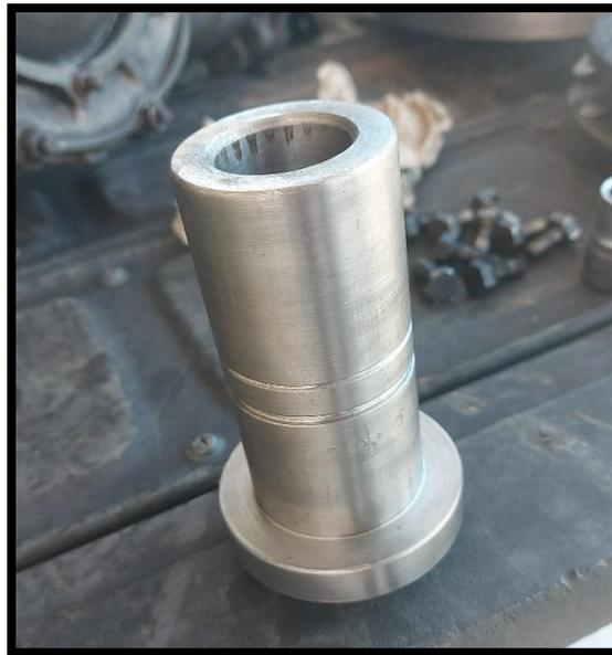
**Figura 4.7.1.1:** Acople Caja Motor
