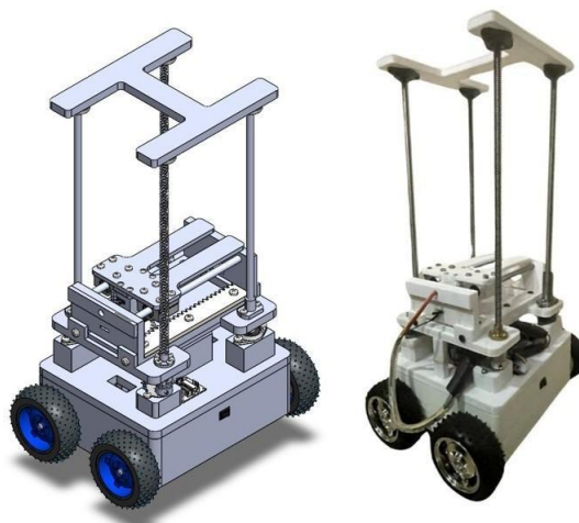
Figure 9. CAD design and implemented prototyping of the robot
