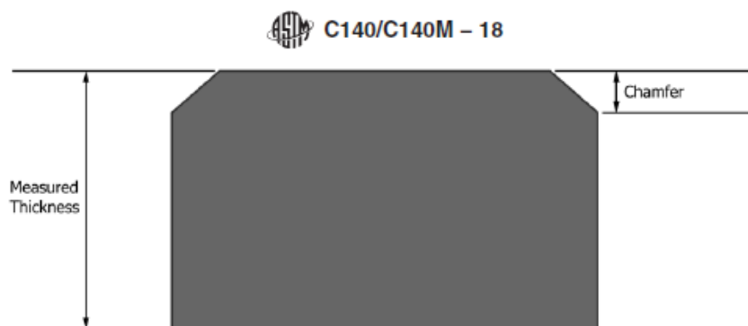
FIG. A4.1 Measuring Thickness of Paver with Chamfer (Section view from end of paver)
