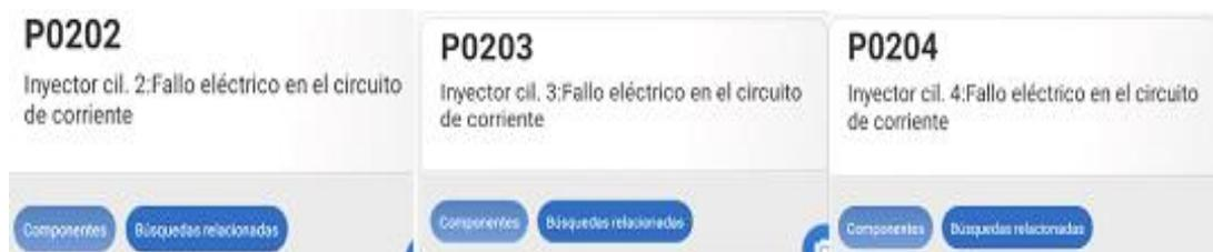
**Figura 45****Borrado de los Códigos de Fallas de los Cilindros**
