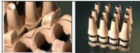
Figure 47. SLS made perforated mould detail for fibre forming (left) and an innovative paper pulp made package for wine bottles (right) (Source: Regale Corp.)
