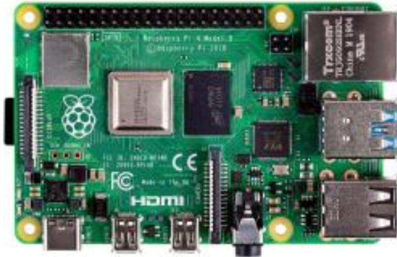
Raspberry Pi 4 Model B is the latest product in the popular Raspberry Pi range of computers. It offers ground-breaking increases in processor speed, multimedia performance, memory, and connectivity compared to the prior-generation Raspberry Pi 3 Model B+, while retaining backwards compatibility and similar power consumption. For the end user, Raspberry Pi 4 Model B provides desktop performance comparable to entry-level x86 PC systems.
