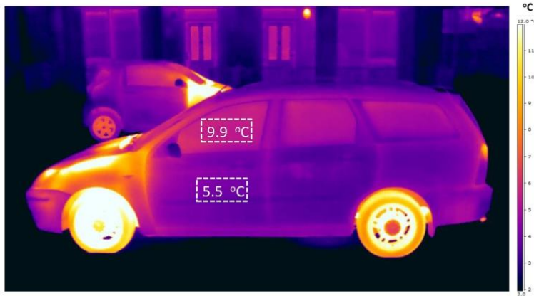
Fig. 4. The infrared image of the tested car during winter with calibrated temperatures based on the measured values from the temperature data logger.
