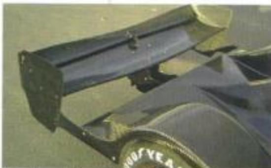
The Dautless rear wing has been staged to work with the flows coming off the car (Courtesy: Dautless Racing)
