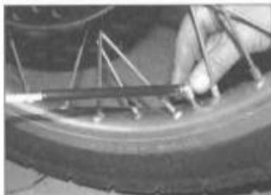
**1** Remove the dust cap from the valve and check the tyre pressures when **cold**. Do not forget to fit the cap after checking the pressure.
