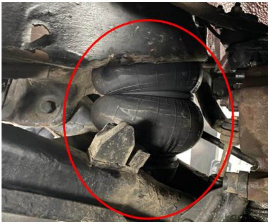
Figura 32 Bolsa de Aire Airmax Instalada
