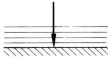
Figure 1.13 Magnetic force: field parallel to the surface
