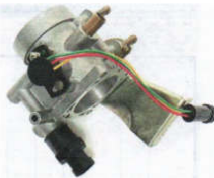
Figure 4.43 Stepper motor and throttle potentiometer on a throttle body
