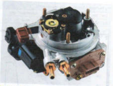
Figure 4.46 Throttle body with a single injector
