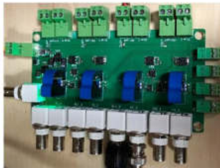
Figure 3. Control and measuring module.
