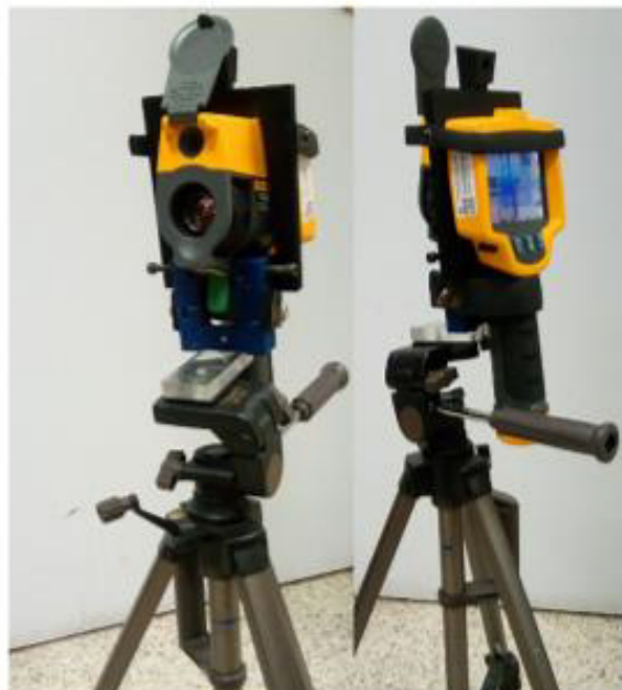
Fig. 2. Infrared thermal camera FLUKE TI32.
