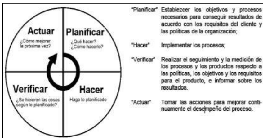
Figura 7. Etapas del ciclo de Deming, ciclo PDCA (Planning, Doing, Check and Act)
