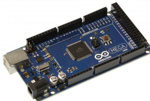
**Figura 51.** Microcontrolador Arduino Mega, [35].
