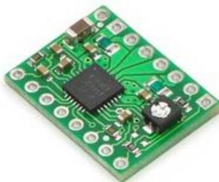
*Figura 3.11: A4988 Stepper Motor Driver Carrier*
