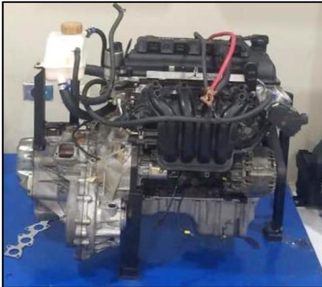
*Figura 2.* Motor 1.4L S-TEC III0
