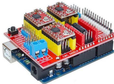
Figura 71 Shield CNC Arduino
