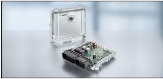
**Figura 2.4** Electronic Diesel Control
