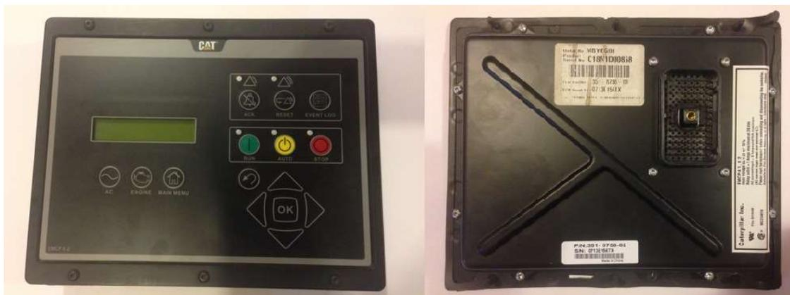
**Figura 131:** Panel de control EMCP 4.2
