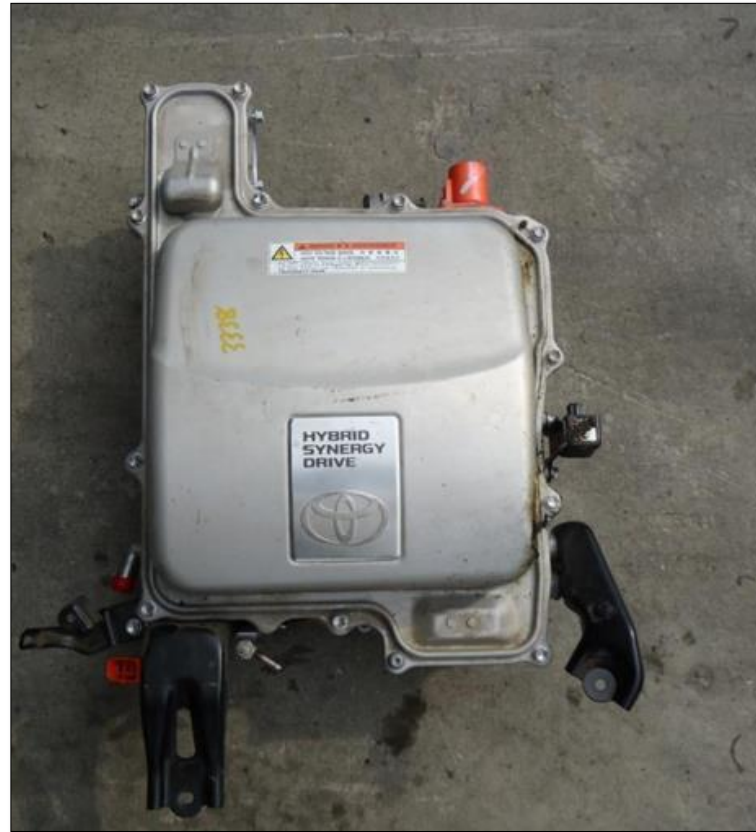
Figura 2.9 Inversor Toyota Prius
