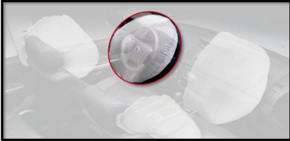
Figura 3.15 Airbag Conductor
