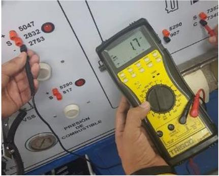
A photograph showing a person's hands using a yellow multimeter to measure a voltage. The black probe is connected to a common ground, and the red probe is connected to pin 7349 on a control panel. The multimeter display shows 1.7. The panel has various pins labeled: 5047, 2832, 2753, 5290, 817, and 7349. There is also a label 'PRESION DE COMBUSTIBLE'.              |
