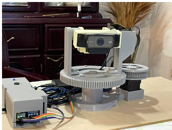
Fig. 17. Physical implementation and final assembly of the mechatronic tracking system.
