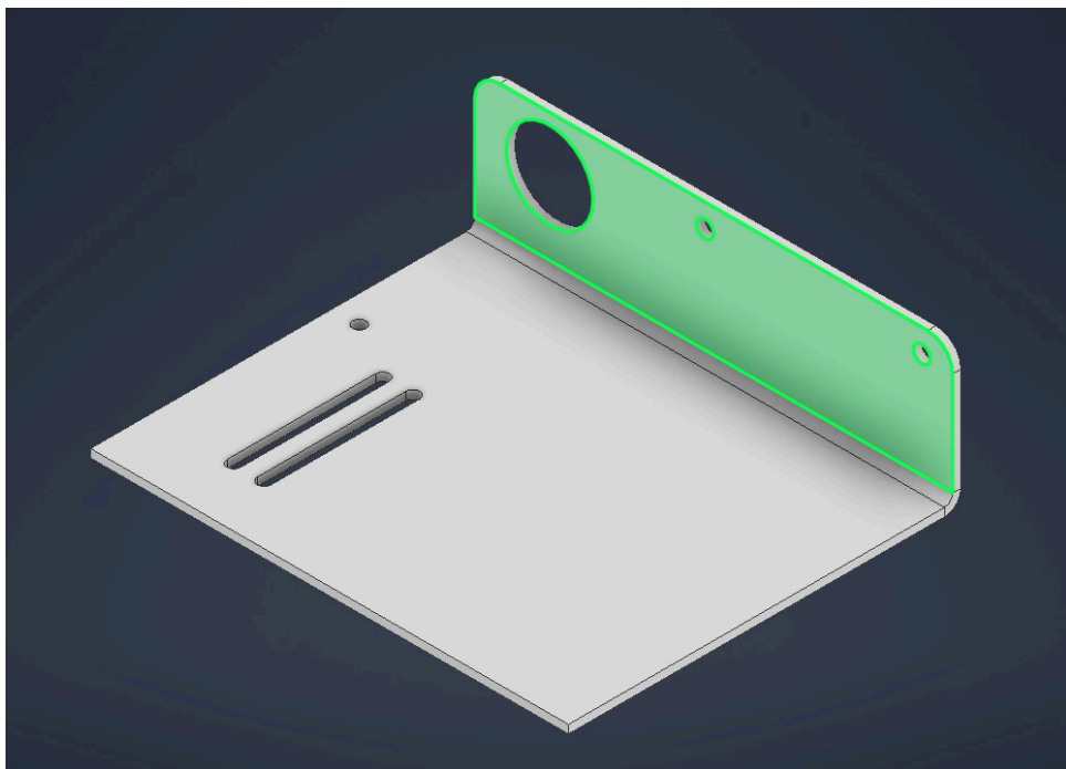
Fig. 4. Detail view of the motor mounting face of the aluminium bracket.
