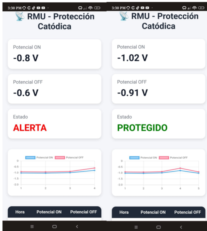
Fig. 19. Remote Viewing on a Cell Phone via a GSM Connection
