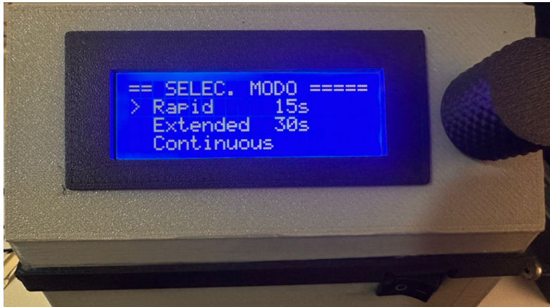
Fig. 13. LCD 20x2 operator interface displaying the active shredding mode and cycle status during a Prototype 2 test.
