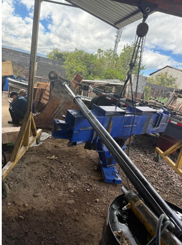
Fig. 13. Second hydraulic cylinder used for the functional validation stage
