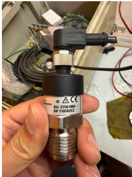
Fig. 8. Industrial pressure transducer used for chamber-pressure measurement
