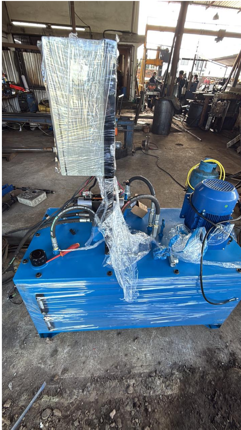
Fig. 10. Automated hydraulic cylinder test bench used for experimental validation
