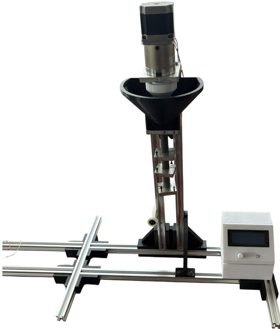
Fig. 11. Extrusion tower and HMI control enclosure.
