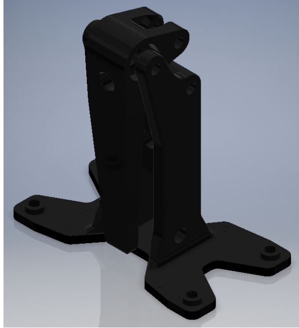
Fig. 5. Lever-based filament diameter measurement system.
