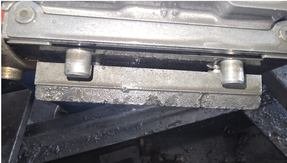
Fig. 14. Fractured honing stone during prototype 1 tests.
