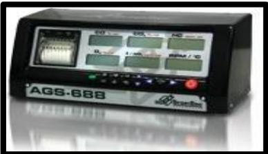
A black rectangular gas analyzer device with a digital display and several buttons. The model number 'AGS-688' is visible on the front panel. | Analizador de gases de escape (vehículos a gasolina). |
