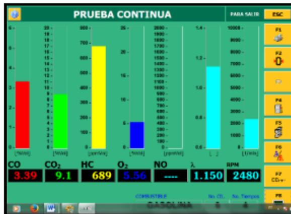
**PRUEBA EN BAJA (RALENTI 800 R.P.M. – 1200R.P.M.)**
