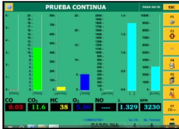
**PRUEBA EN BAJA (RALENTI 800 R.P.M. – 1200R.P.M.)**
