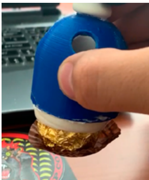
Figure 6. Vacuum grip using salt.
