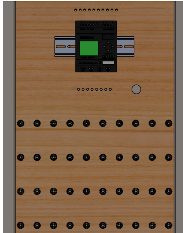
Figure 7: View of the connection board where the terminal blocks are located.
