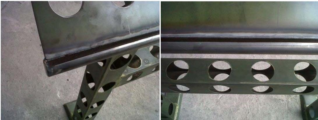
**Figura 4.38 Canal recolector de aceite.<sup>51</sup>**
