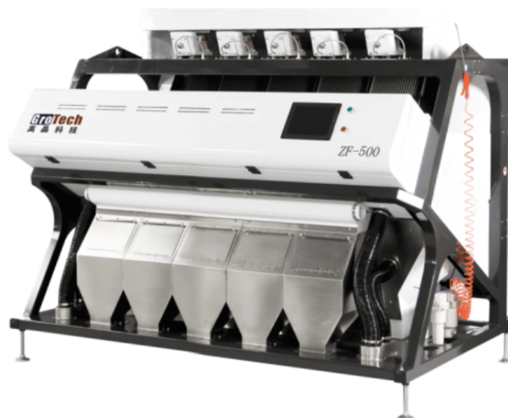
Figura 11. GROTECH Multifunction color sorte [20].
