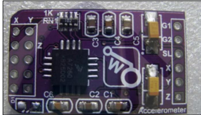
The MMA7260Q low cost capacitive micromachined accelerometer features signal conditioning, a 1-pole low pass filter, temperature compensation and g-Select which allows for the selection among 4 sensitivities. Zero-g offset full scale span and filter cut-off are factory set and require no external devices. Includes a Sleep Mode that makes it ideal for handheld battery powered electronics.
