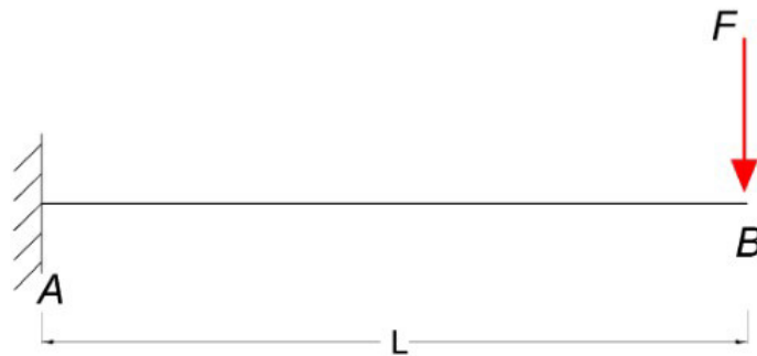
Figure 5. Free body diagram of the cantilever beam with single load at end
