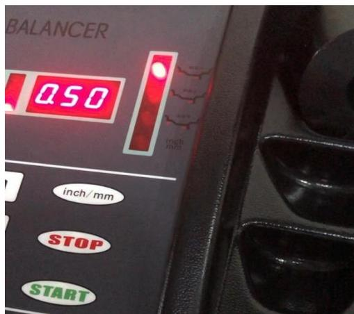
**Figura 74***Colocación de Contrapesos en la Parte Interior de la Llanta*
