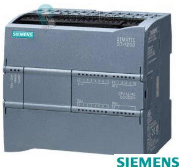
Figura 73. PLC Siemens S7-1200, Modelo 1214C [20].
