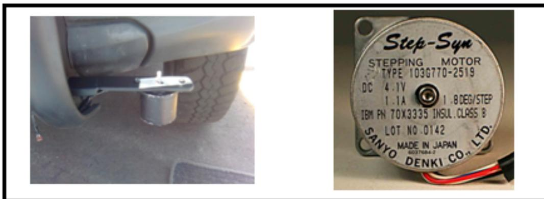
**Figura 3.18** Motor de paso Sanyo Denki Co.
