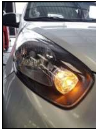
Figura 2.9 Luces de parking o emergencia
