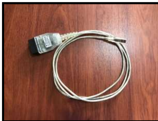
Figura 32. Mongoose Interfase (TAEET Electronics)
