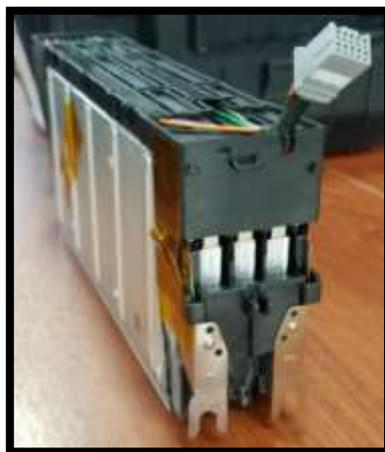
**Figura 60.** Block de celdas
