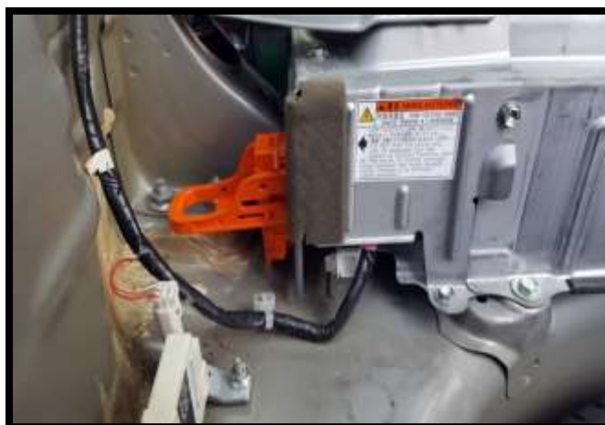
Figura 59. Accionamiento de Jumper de seguridad hacia atrás ( www.hybridcars.com/hybrid-owners-reconditioning-your-battery-is-a-possibility/ )
