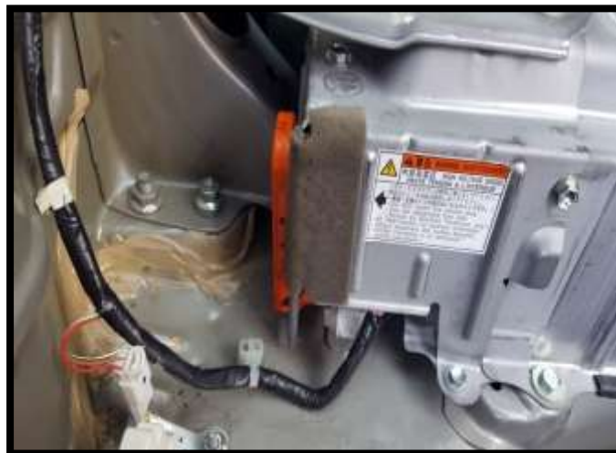
Figura 58. Interruptor con fusible o Jumper de seguridad (color naranja) ( www.hybridcars.com/hybrid-owners-reconditioning-your-battery-is-a-possibility/ )
