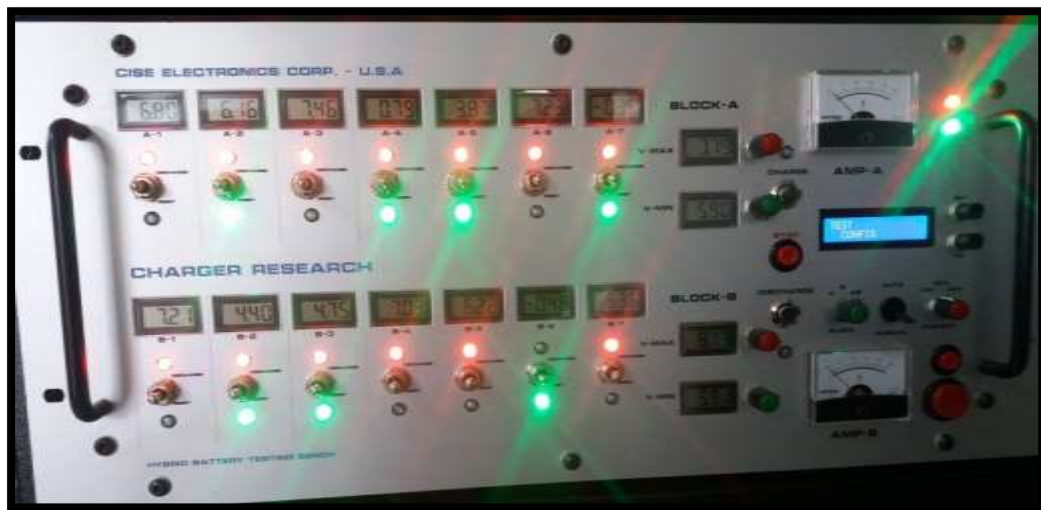
Figura 48. Corriente de descarga de 1 Amp (Cise Electronics)
