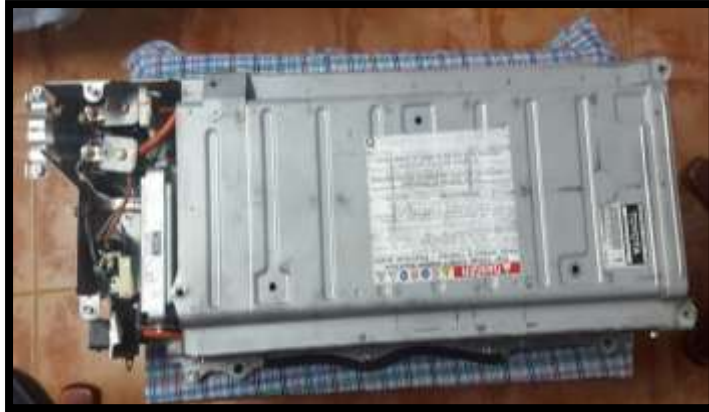
Figura 61. Batería híbrida desmontada I ( www.hybridcars.com/hybrid-owners-reconditioning-your-battery-is-a-possibility/ )
