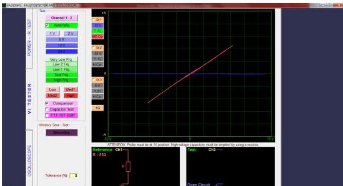
**Figura 66.** Curva V/I conector del sensor MAF a la ECU, terminal #2.
