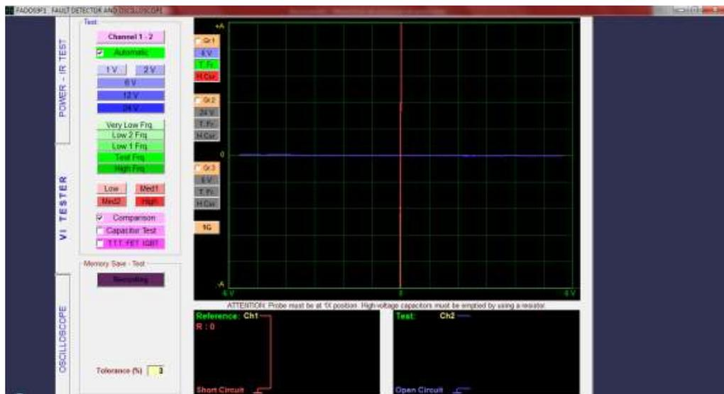
**Figura 70.** Curva V/I conector del sensor O2 a la ECU, terminal #1.
