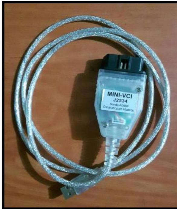
**Figura 20. Interfaz OBDII MINI-VCI J2534.**
